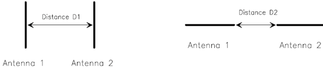
Figure 6.1 Distance between antennas (top view)
