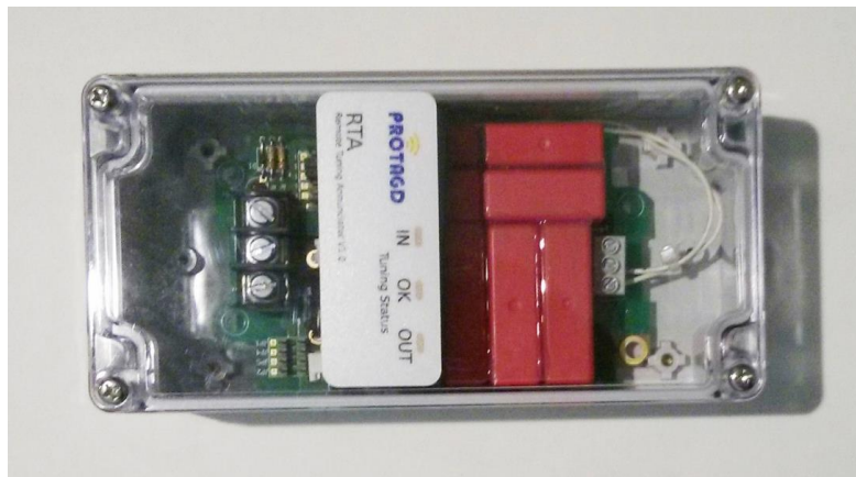
Figure 3.3 PRDRTA installed into Antenna tuning box
